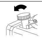
Replace and tighten dipstick. Remove and check oil level.
